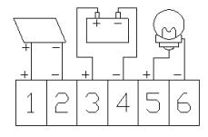
2. Connect the "+", "- " Poles of the solar panel to the relevant terminal of the controller (the first one and the second one) firmly and correctly.
